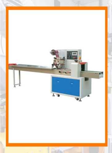
In case of Horizontal Form Fill Seal Machines, the machine operation is Intermittent. Plastic Laminated Film is drawn off a supply reel by a pair of rollers. The Reel passes over a folding plough which folds it into half.
