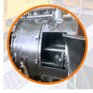
The mixer is designed for heavy duty blending of both dry and wet material. Plough shape shovels mounted on a central shaft with its sharp ends easily penetrate through the dense powder and thick pasty mass. Extra shear can be attained by adding side mounted choppers.
